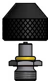
Model of valve stem 7/8" 14 UNF (B)
