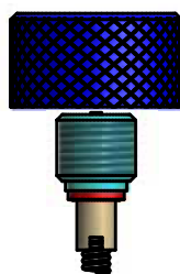
Model of valve stem 7/8" 14 UNF (C)
